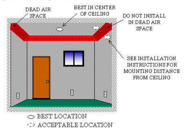
The smoke alarm must be mounted on an electrical box. When the box is cut into the ceiling or wall, the opening must be flush with the ceiling or wall surface. You should be able to see the electrical box opening when the detector is detached from the box. You MUST use listed wire nuts for any wire splices- twisting the wires together and taping the bare wires is not acceptable!
