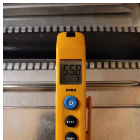
supply temp - temp drop of approximately 16 degrees (acceptable)
