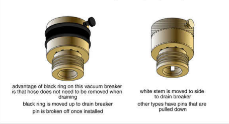
Hose bibb vacuum breakers (draining required)
