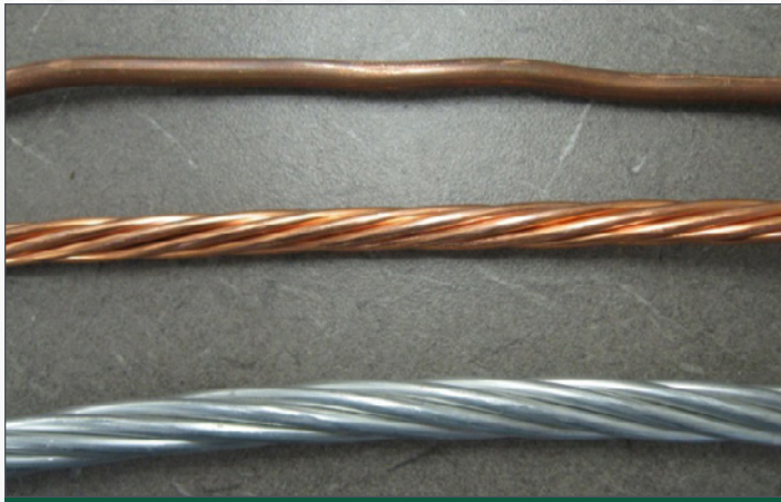
Example of Bonding Conductor
